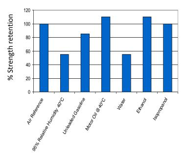
Specimens were immersed for 1000 hours at 22°C (unless otherwise stated)
