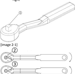
4. To release the ratchet feed handle from the machine, press the release button on the ratchet feed handle (image 2-2, ② and image 2-3, ②) and pull it away from the machine
