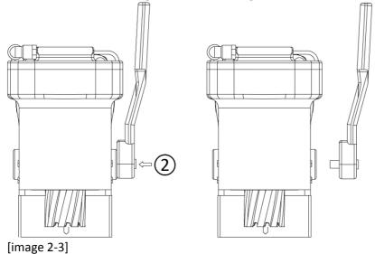
5. It is possible to position the ratchet feed handle on either side of the machine (image 2-4). Method of fitting and releasing (steps 1. to 4.) is always the same.
