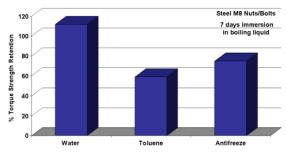
This product is not recommended for use in contact with steam, strong oxidizing materials and polar solvents although will withstand a solvent wash without any bond strength deterioration.
