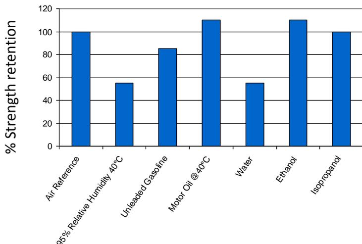
Specimens were immersed for 1000 hours at 22°C (unless otherwise stated).
