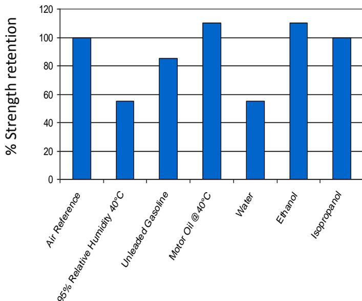
Specimens were immersed for 1000 hours at 22°C (unless otherwise stated)
