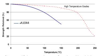
"Hot strength" shear strength tests performed on mild steel. 24hr cure at room temperature and conditioned to pull temperature for 30 minutes before testing.
