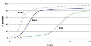
Cure times are typical at 23°C. Copper and its alloys will follow the faster cure while oxidised or passivated surfaces like stainless steel will tend towards the slower curve. Lower temperatures or large gaps will tend to extend the cure time. To reduce the cure time the use of Permabond A905, ASC10, or heat can be considered.
