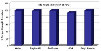
This product is not recommended for use in contact with steam, strong oxidizing materials and polar solvents although will withstand a solvent wash without any bond strength deterioration.
